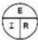
Figure 1-8.—Ohm's law in diagram form.
